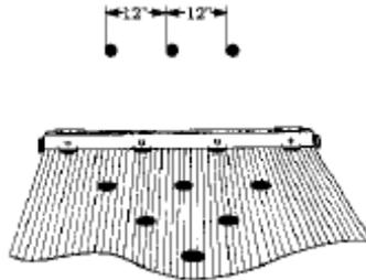
4. If any pin spots are not exactly 12 inches from each adjacent spot, mark the "No" box on the form [Page 2, Item 5] and write details under "Remarks" (Make a diagram on a separate sheet of paper, if needed, to describe non-complying measurements.)
