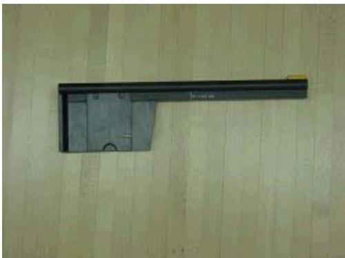
*Gutter, Pit and Pit Cushion Checking Gauge*
