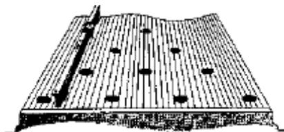
2. Be sure that the level is flat on the deck surface, and not lifted by a splinter or other obstacle on the deck. (If level has feet, this is no problem.)
