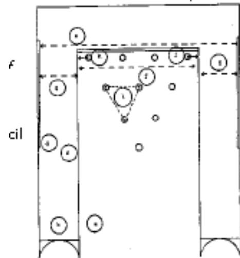
The final diagram shows a useful sequence for the remaining pit end measurements, and includes the use of the Pit and Gutter Gauge and the Bowling Lane Gauge, and concludes with your checking the accuracy of the pin spotting.
